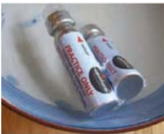
The float test. The spent canister on the left floats, telling me (without test spraying) that it is empty.
